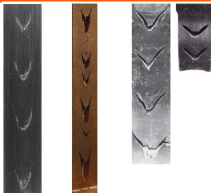
Sections showing chevron crack
