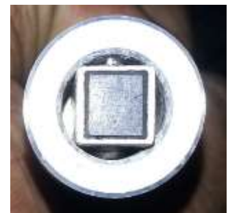
16 element PAUT probe in adapter casing
