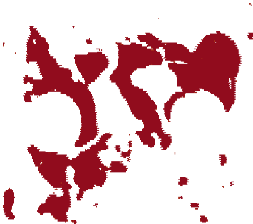
C-scan image showing the unbonded region (in red) of the brazed joint in a bus bar assembly
