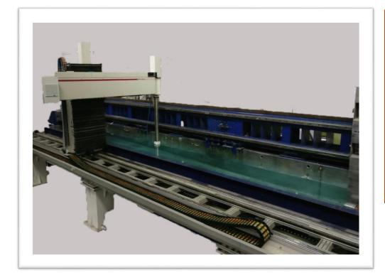
Automated Phased Array Immersion Ultrasonic Testing System for Inspection of GUN Barrel, Breech Ring and Casings
