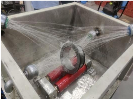
The sample is washed in pre tank
