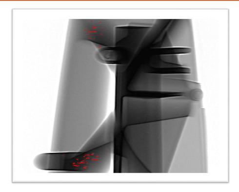
**ROBOTIC ARM BASED** AUTOMATED DIGITAL X-RAY INSPECTION SYSTEM FOR **ALUMINUM CASTINGS** WITH AUTOMATIC **DEFECT RECOGNITION** (ADR)
