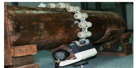
The beauty of a technology is when it's not localized to a particular application. The same technology is employed for different applications like Tank Annular Plate scanning, Railway Feet weld inspection etc . For pipes another application is when we are generating axial HOMC instead of circumferential HOMC. There
