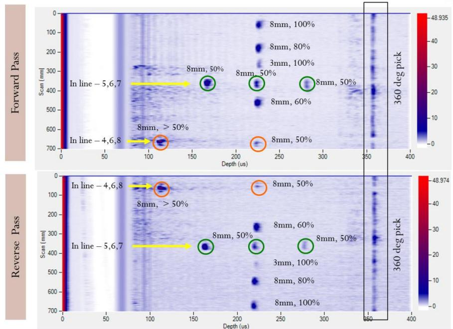
Inspection B Scan Images showing defects. Forward pass is inspection in one direction and reverse pass is inspection in the reverse. Both conform the repeatability of scans.
